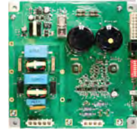
EPC Control Board
